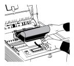
4. Pull out the protect sheet of paper from the image drum cartridge.
